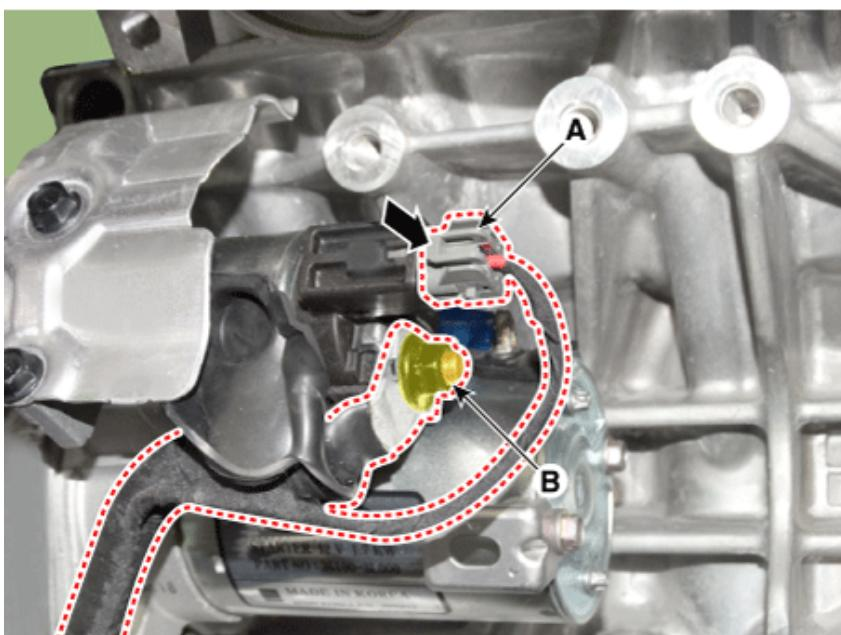
17. Remove the starter (A) after loosening the mounting bolts (B).
